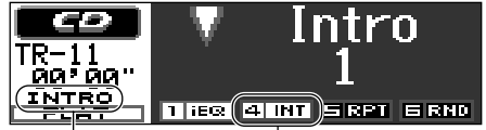
INTRO indicator INT indicator (See the following table.) Ex.: When you select "Intro 1."
