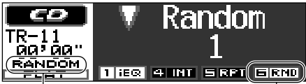
RANDOM indicator RND indicator (See the following table.) Ex.: When you select "Random 1."
