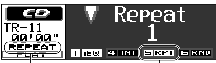
REPEAT indicator RPT indicator (See the following table.) Ex.: When you select "Repeat 1."
